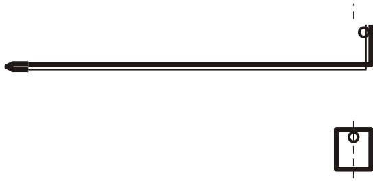
Fig. 10 — The bracket, drawn from the part drawing. Side elevation above, wall plate seen face on below.
